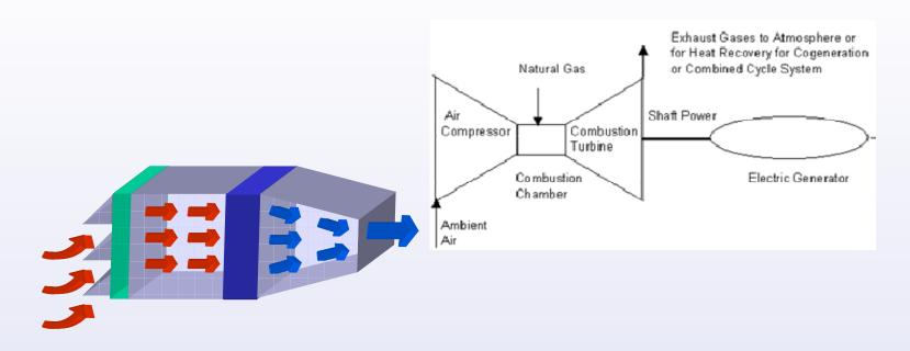
• Cooling the inlet air before or during compression in the compressor that supplies high-pressure compressed air to the combustor of the CT
