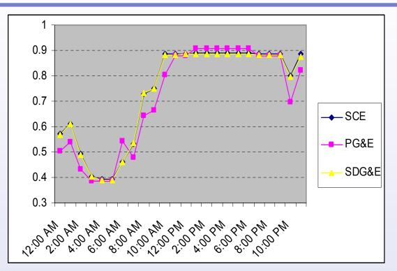
Y-Axis Unit: CO<sub>2</sub> Emissions, Lbs/kWh
