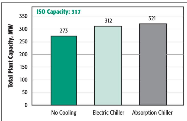
Figure 2. Effect of Chiller Technology on Net Power Output
