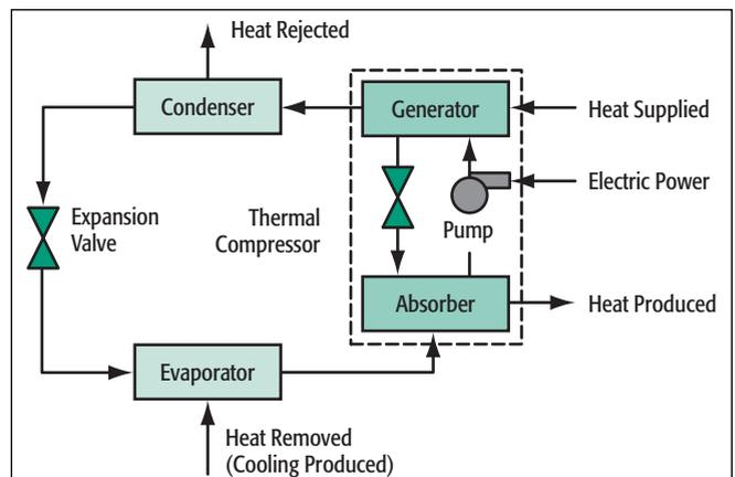
Figure 1. Process Schematic of a Single-Effect Absorption Chiller
