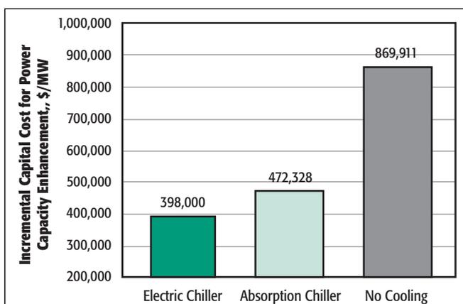
Figure 4. Effect of Chiller Technology on Capital Cost for Incremental Plant Capacity Enhancement
