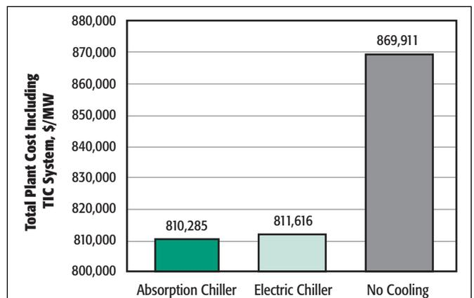
Figure 3. Effect of Chiller Technology on Total Plant Investment
